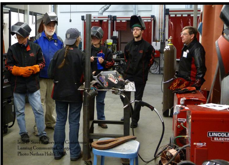
LCC instructors Cathie Lindquist (center left) and Bill Eggleston (right) prepare to demonstrate pad welding (SMAW and FCAW) for section loss (historic eye bar shown in foreground)
