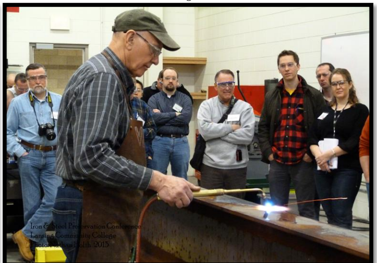
Vern Mesler demonstrates heat straightening
