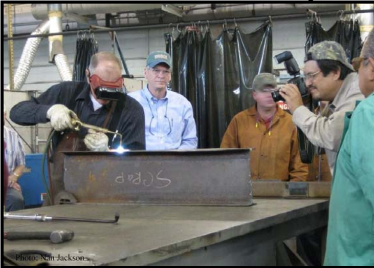
Flame straightening methods of Joseph Holt demonstrated
