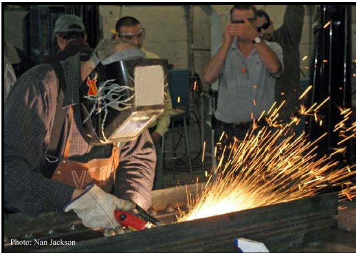
Vern Mesler removes rivets using Air Carbon-Arc Process
