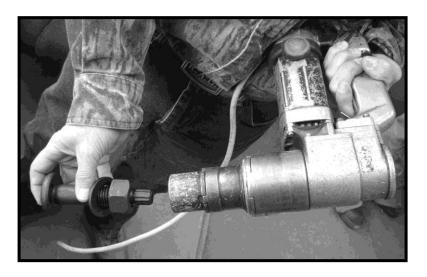
Button head tension control bolt with specialized wrench
