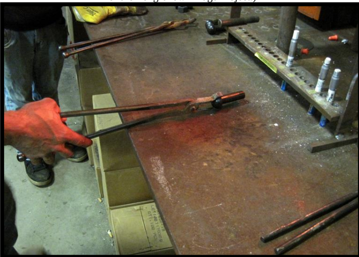
Employee at Atlantic prepares to heat a rivet. Rivets were produced at Chicago Fasteners to ASTM Standard Specification for Rivets, Steel, Structural, A502-03
