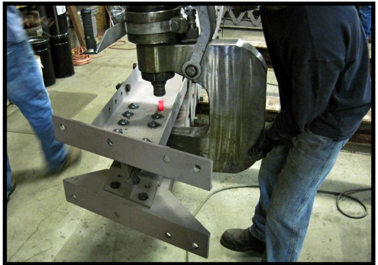
Hydraulic riveter positioned to drive heated rivet on a vertical post at Atlantic. Imported and retrofitted by Steve Howell, Ballard Forge, Seattle, Washington
