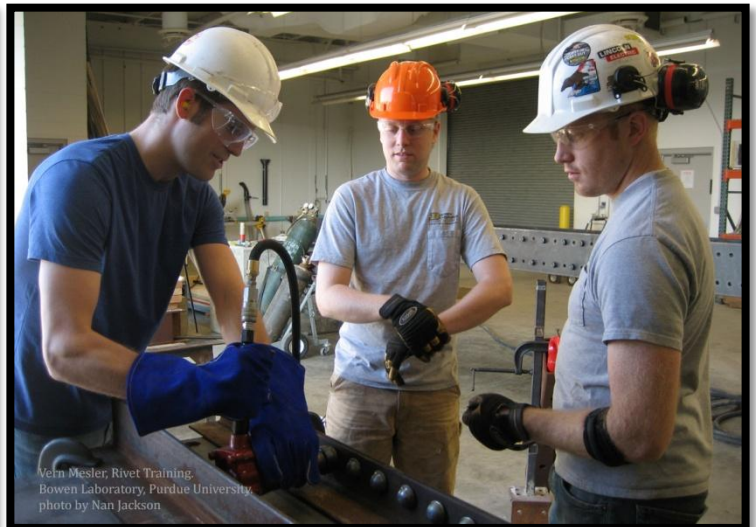
Brian Richter Purdue M.S. student practices using the holder-on, while Sherman and Hebdon look on.
