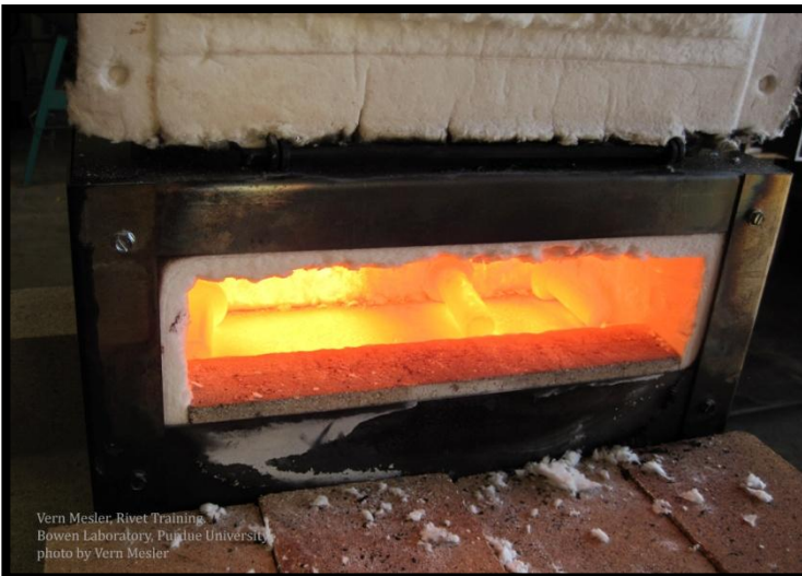
Propane forge heats rivets to 1900 - 2000 degrees F.
