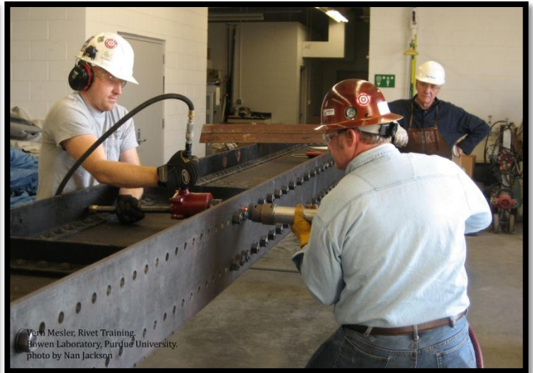
Hebdon sets holder-on; Robert Connor, Purdue Associate Professor of Civil Engineering, drives rivet.
