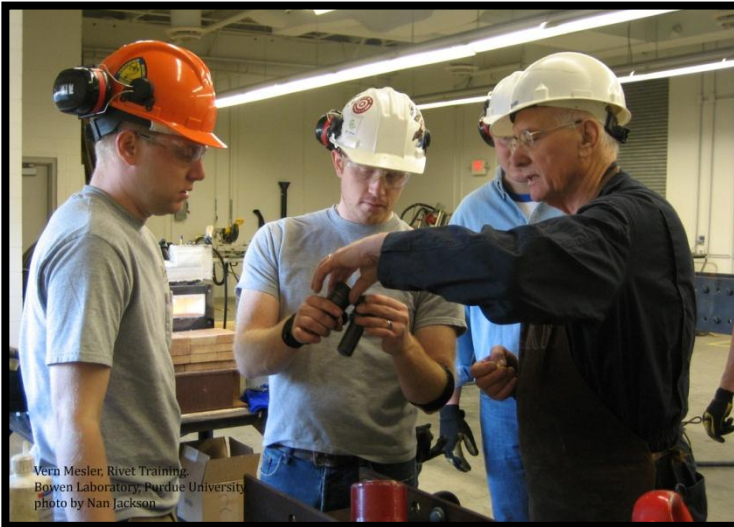
Sherman, Hebdon and Vern Mesler inspect rivet snaps
