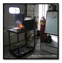
Temperature gauge is attached to the forge and a clock is handy for recording temperatures at one-minute intervals after the rivets are placed inside.
