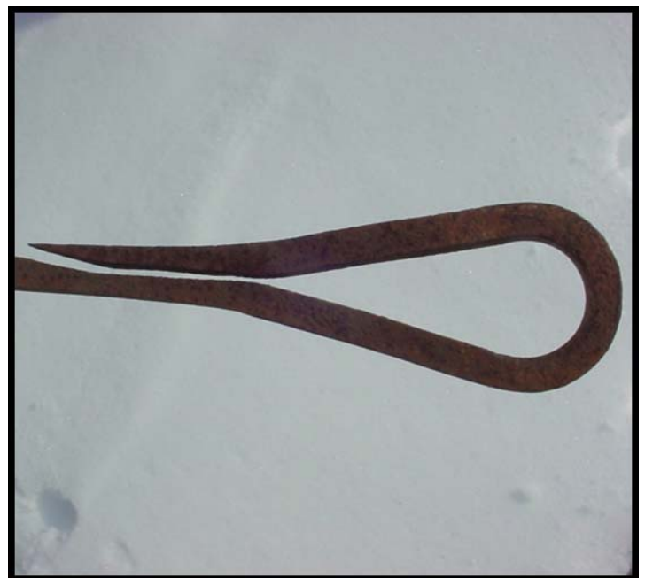
Photo 12: Broken forge weld from a Michigan Historic Bridge
