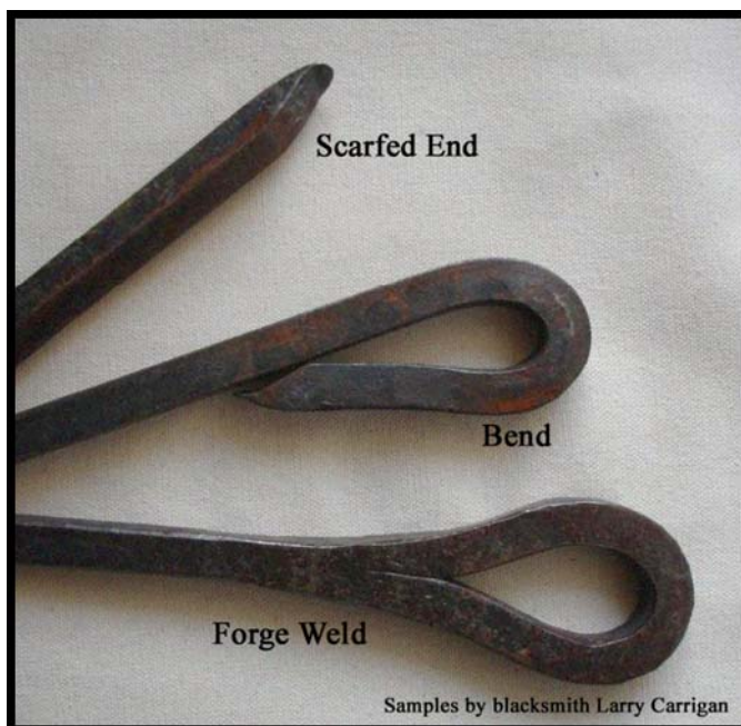
Photo 11: Forge Welding of Loop Eyebars
