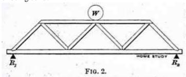
A metal compression member, of nearly any form, can readily be made to resist a certain amount of tension also. But members designed to resist tension only, are not generally capable of resisting compression. When it is desirable that a tension member shall resist a certain amount of compression also, it is generally necessary to modify the form of the member.
