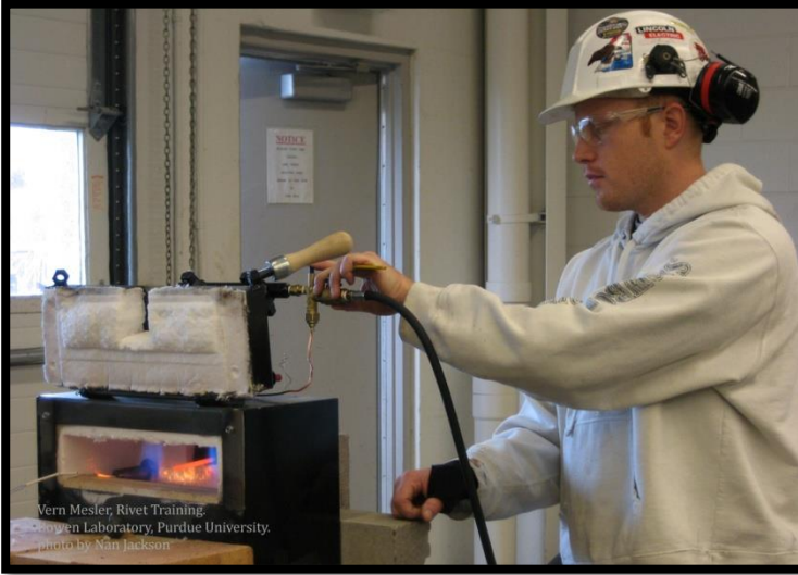
Matt Hebdon, Purdue Ph.D. research assistant, adjusts propane forge in preparation for riveting.
