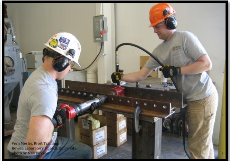
Hebdon drives 7/8" rivets with a #80 Boyer rivet hammer. Sherman positions a holder-on which keeps the hot rivet in place.
