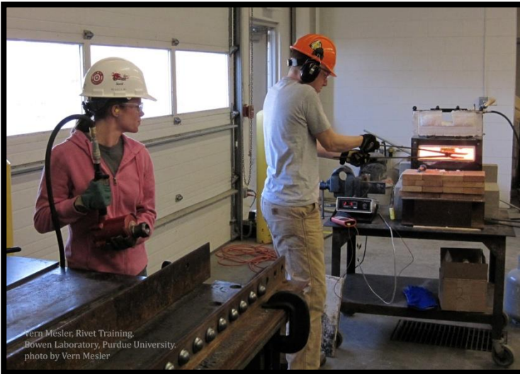
Teresa Washeleski, Purdue M.S. student, with holder-on; Sherman heats rivets.
