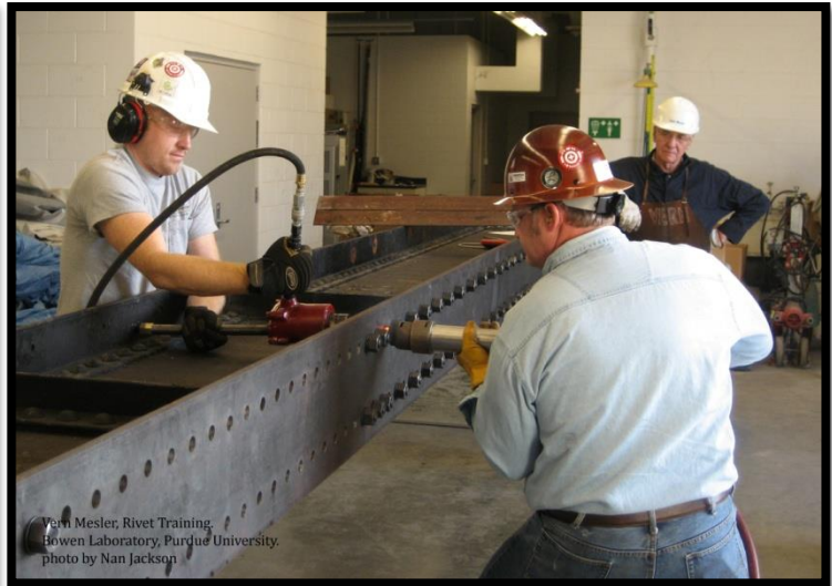
Hebdon sets holder-on; , drives rivet.
