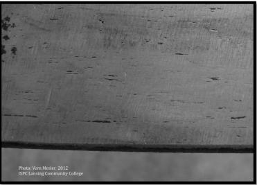
Clear enamel brings out surface detail; wrought iron siliceous slag is clearly visible.
