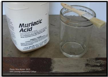
With a brush, apply to the heated surface a solution of 5 parts water and one part muriatic acid. Apply liberally. Wash with water; air cool and dry.
