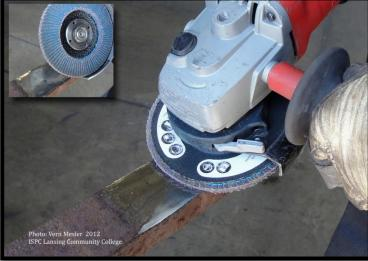
Replace the grinding wheel with a 60 grit (or finer) 4" abrasive flap disk. Polish in one direction (the same direction as the grinding) until most of the grind marks have been removed.
