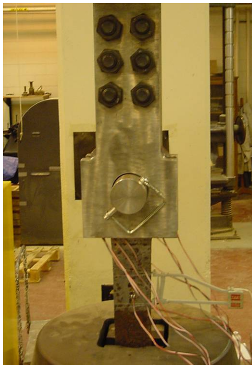
Figure 3.23 Eyebar Connection in MTS Machine with Added Setup before Testing
