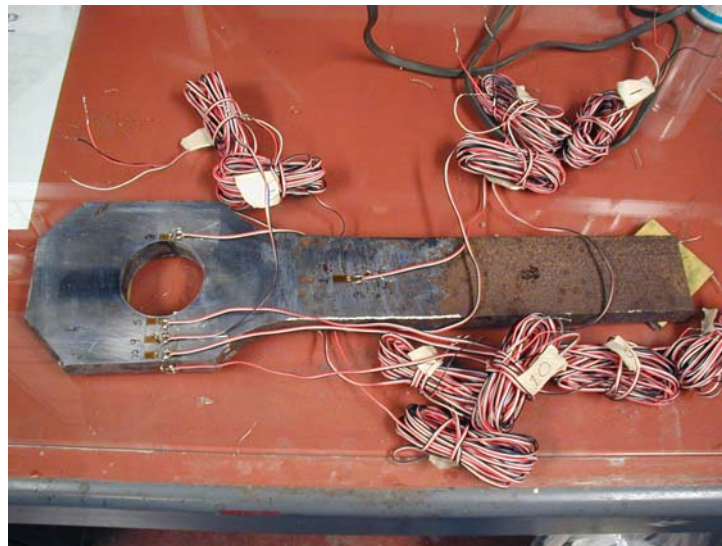
Figure C.20 Eyebar End Connection after Strain Gages were Attached
