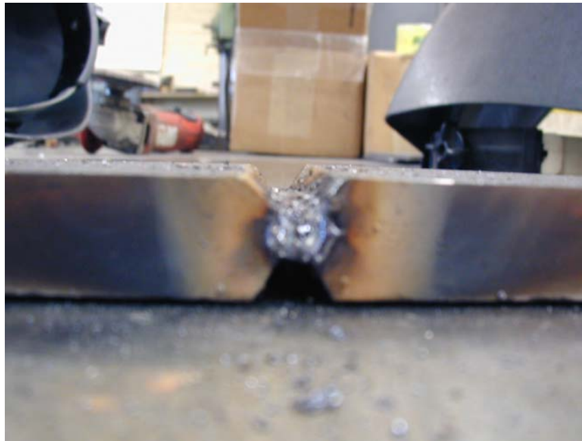
Figure D.2 Weld Joint After Initial Root Pass
