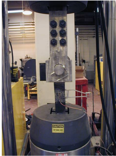
Figure 3.35 Front View of Eyebar B in Testing Machine with Extensometer Attached
