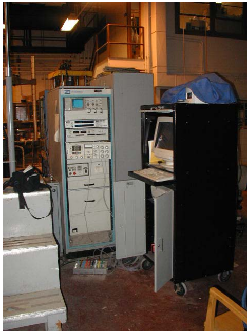
Figure C.14 Controller and Function Generator of the 220-kip MTS Four-pole Servo-Hydraulic Testing Machine Along With the Data Acquisition Center (Scanners and Computer)
