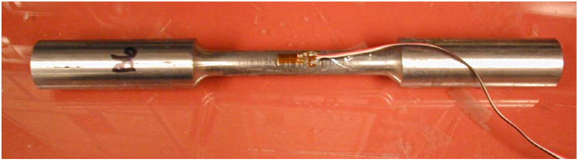
Figure 3.13 Round Tensile Testing Specimen
