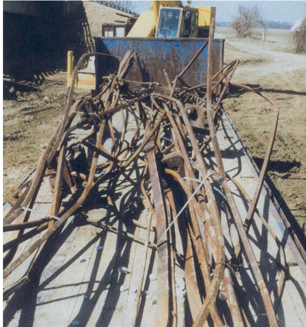
Figure 5.13 Bent and Damaged Members from the Bell Ford Bridge
