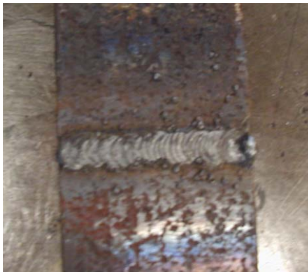
Figure D.5 Completed Weld Before Surface Grinding
