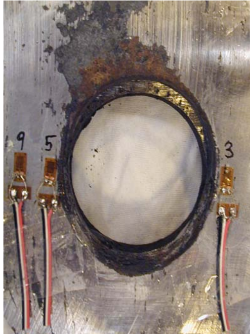
Figure 4.25 Elongation of Hole in Eye Connection after Testing to Failure
