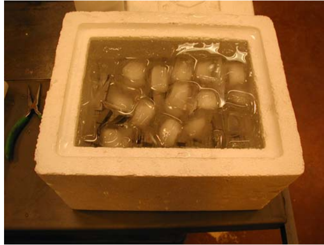
Figure C.19 Cooling Bath with Suspended Charpy Impact Specimens after Water and Ice is Added
