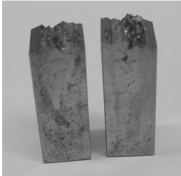
Figure 4.22 Slip Plane Fracture of Charpy Impact Specimen (T Type)
