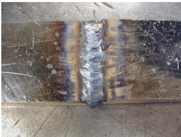
Figure C.10 Finished Weld of Testing Specimen before Surface Grinding
