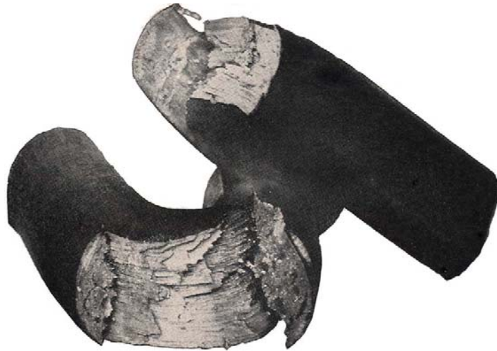
Figure 1.2 Picture Showing Fibrous Nature of Wrought Iron. (Aston, 1949)
