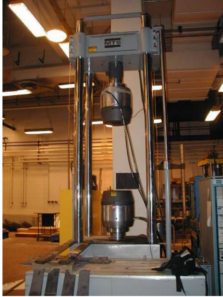
Figure C.13 Grips of the 220-kip MTS Four-pole Servo-Hydraulic Testing Machine
