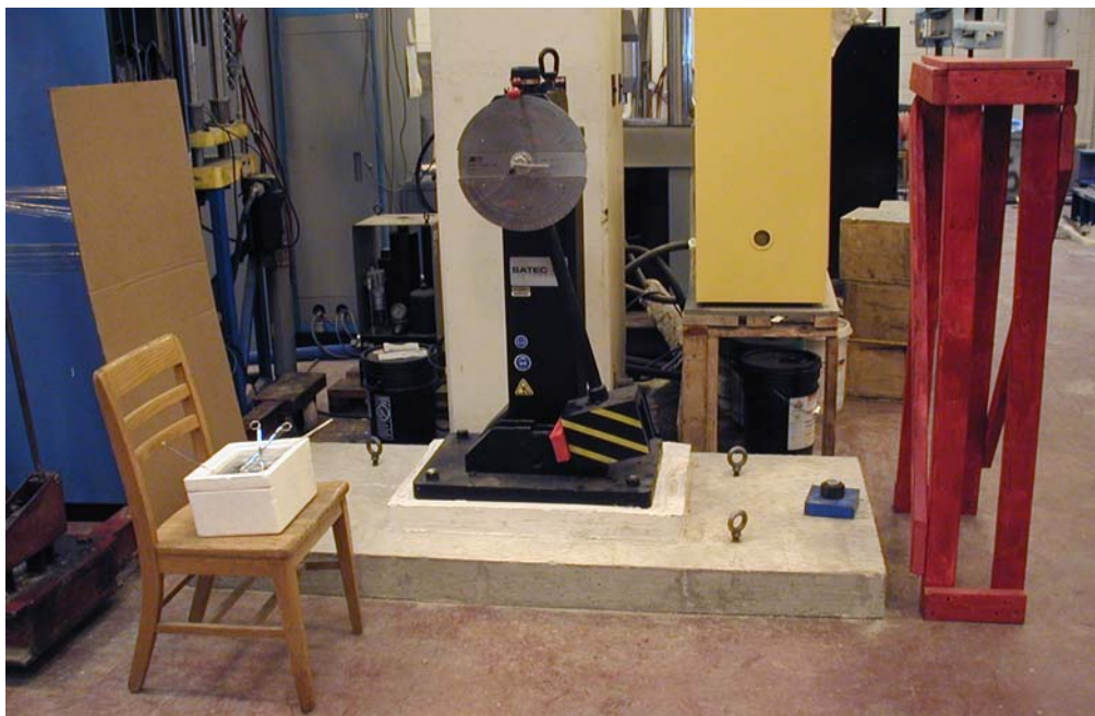
Figure C.17 SATEC Impact Testing Machine Along with Cooling Bath Used in Charpy Impact Testing
